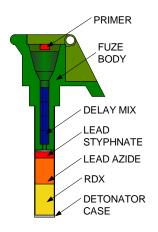
Figure 1: M213 Grenade Fuze (spoon and hammer not pictured)
