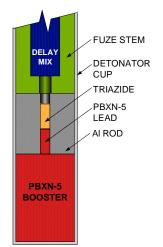
Figure 6: C70 cup loaded with primary and PBXN-5
