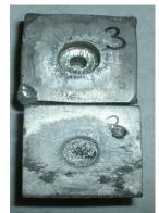
Figure4: Functioned fixture loaded with EDF-2/Cyanuric Triazide.
